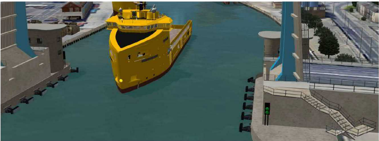
Figure 8.2: Run 01, Inbound PSV entering bridge opening, 16 minutes, 14m to E knuckle
