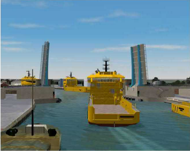
Figure 8.38: Run 09: PSV about 40m from bridge Source: HR Wallingford Ship Simulation System
