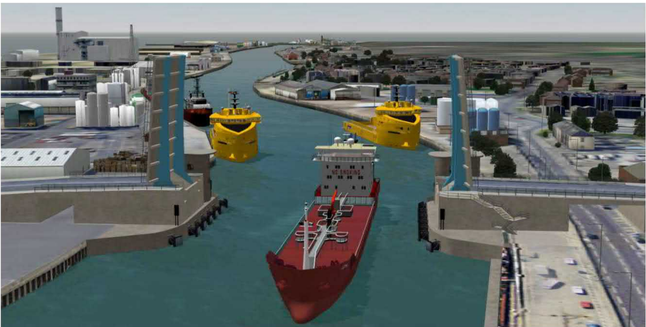
Figure 8.49: Run 15: Ship better aligned in bridge opening
