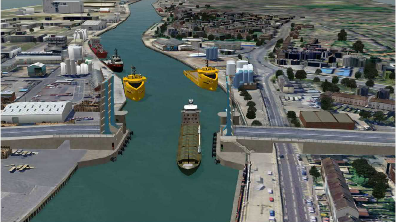
Figure 8.71: Run 33: Outbound Fischland with 6m clearance to eastern knuckle
