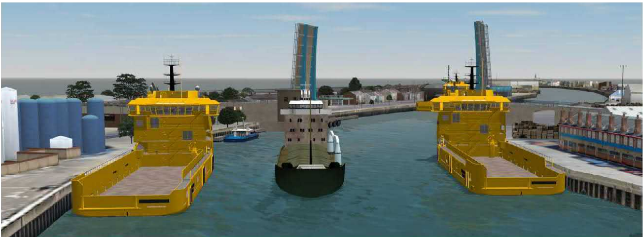
Figure 8.56: Run 32: Inbound Fischland stern first approach to bridge Source: HR Wallingford Ship Simulation System
