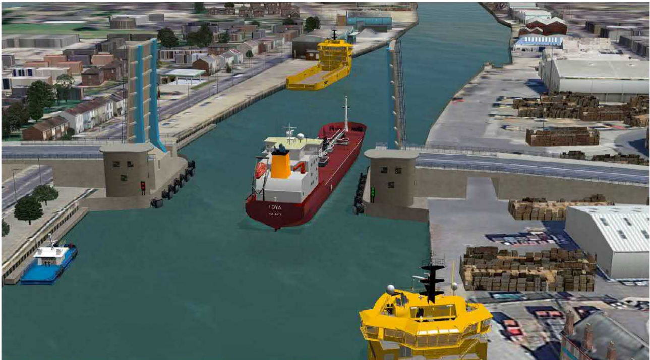
Figure 8.50: Run 24: 4m minimum clearance to east knuckle
